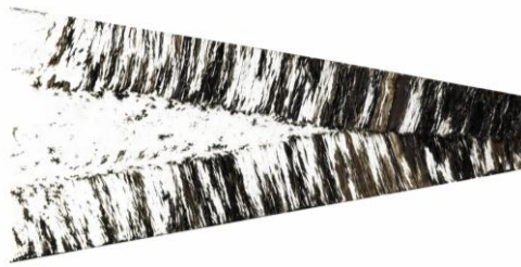
Fig. 5. Microstructure ( \times 300 ) of steel, obtained from wedge-shaped castings
